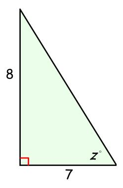
The inverse operation of taking the tangent of the angle is taking the INVERSE tangent of a ratio. On your calculator, you hit the "2<sup>nd</sup>" function button first, then the "TAN" button.
