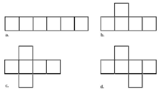
The net is useful to determine surface area, because we reduce the problem to finding the area of the 2-Dimensional solid. We can subdivide the figure in squares, rectangles, triangles, or any other figure for which we know the area formula!!!
