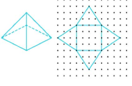
The surface area is the sum of the areas of the 4 congruent triangles and the square base. We can count the dots, each representing one unit, to determine the required side lengths:
